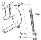
5) Clean spray tip and filter with a soft-bristled brush and the appropriate cleaning solution. Be sure to remove and clean the washer and saddle seat located in the rear of the spray tip assembly.
