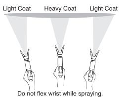
TIP: The spray gun should be triggered by turning it on and off with each stroke. Do not trigger the gun during the middle of a stroke. This will result in an uneven spray and splotchy coverage.
