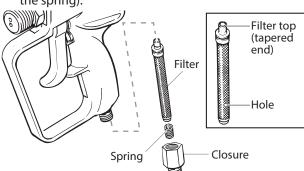
3) Remove the filter from the spray gun housing and clean with the appropriate cleaning solution (warm, soapy water)
