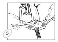
Thread the other end of the hose to the spray gun. Hold the gun with one adjustable wrench, and tighten the hose nut with the other.
