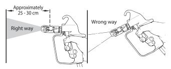
TIP: Keep the spray gun at right angles to the surface. This means moving your entire arm back and forth rather than just flexing your wrist.
