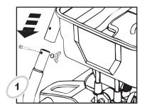
Place the handle over the unit frame. Insert the bolts and tighten the wing nuts over the lock washers.
