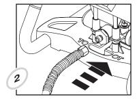
Thread one end of the high pressure spray hose to the outlet valve.
